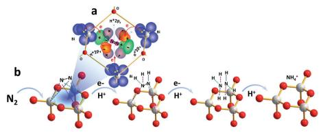
Fig. 6 Possible pathway for  $N_2$  activation and hydrogenation on the BiO catalyst. (a) Schematic electron donation from the lone pairs of three Bi atoms to the three unoccupied anti-bonding orbitals  $(\sigma^*2p_x, \pi^*2p_y)$  of the  $N_2$  molecule, forming a  $1N_2-3Bi(II)$  side-on bond structure. (b) The whole  $N_2$  activation and reduction process on the BiO catalyst.
