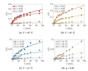
Fig. 4 Swelling of pre-made polymer networks of four representative conversions  $\chi$  at (a) 65 °C, (b) 45 °C, (c) 21 °C and (d) at a single conversion  $\chi$  = 0.85 and three temperatures. Each panel shows the evolution of the strain  $\varepsilon(t) = h(t)/h(0) - 1$ , where  $h(0) = 150 \mu m$ . Symbols and solid lines respectively correspond to experimental data and numerical fits of the reduced model (18).
