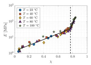
Fig. 3 The dependence of the elastic modulus E on the monomer-topolymer conversion fraction  $\chi$  at different temperatures. The dashed line denotes the glass transition.
