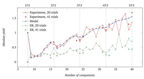
Fig. 15 Results for the systems with N = 8 (45°) sectors per circular target structure: comparison of model-predicted and experimental absolute assembly yield, including error bounds for 20 and 41 trials. Vertical dotted lines extend the markers on the x-axis for the fully formed target structures. See also Fig. 4.
