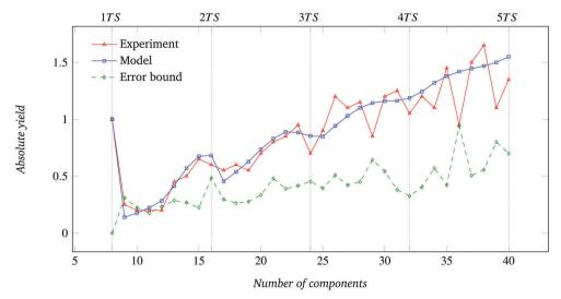
Fig. 4 Results for the systems with N = 8 (45°) sectors per circular target structure: absolute assembly yield for experiments with physical system, absolute assembly yield for analytical model, and 95% error bound. Vertical dotted lines extend the markers on the x-axis for the fully formed target structures. Experimental data collected over 20 trials per condition.
