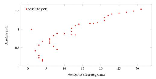
Fig. 16 Scatter plot of absolute assembly yield as a function of possible absorbing states for the system with  $N = 8 (45^{\circ})$  sectors per circular target structure. Experimental yield values are from 20 trials (refer to Fig. 4 and 5).
