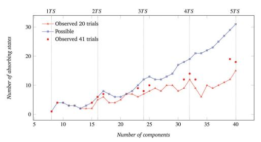
Fig. 5 Number of possible and of observed absorbing states as a function of the number of components for the system of Fig. 4.
