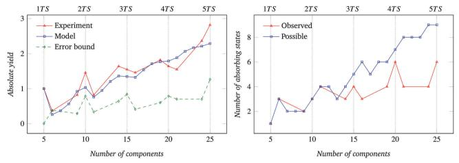
Fig. 8 Results for the systems with N = 5 (72°) sectors per circular target structure: (left) absolute assembly yield for experiments with physical system, absolute assembly yield for analytical model, and 95% error bound. Vertical dotted lines extend the markers on the x-axis for the fully formed target structures. Experimental data collected over 11 trials per condition. (right) Number of possible and of observed absorbing states as a function of the number of components.
