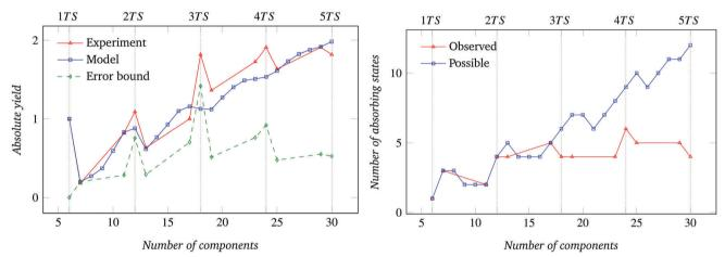
Fig. 7 Results for the systems with  $N = 6 (60^{\circ})$  sectors per circular target structure: (left) absolute assembly yield for experiments with physical system, absolute assembly yield for analytical model, and 95% error bound. Vertical dotted lines extend the markers on the x-axis for the fully formed target structures. Experimental data collected over 11 trials per condition. (right) Number of possible and of observed absorbing states as a function of the number of components.
