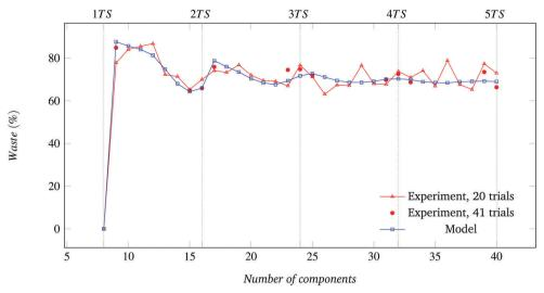
Waste, i.e., relative fraction of components not assembled into target structures, for the system of Fig. 4.
