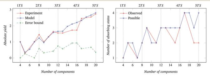
Fig. 9 Results for systems with N = 4 (90°) sectors per circular target structure: (left) absolute assembly yield for experiments with physical system, absolute assembly yield for analytical model, and 95% error bound. Vertical dotted lines extend the markers on the x-axis for the fully formed target structures. Experimental data collected over 11 trials per condition. (right) Number of possible and of observed absorbing states a function of the number of components.
