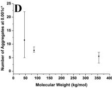
Fig. 12 Graphs showing how molecular weight affects the number of polymer aggregates on a specific surface area of mica at varying concentrations. Each graph presents the average values and has bars which indicate the range of values. (A) 1c\*, (B) 0.1c\*, (C) 0.01c\* (D) 0.001c\*.
