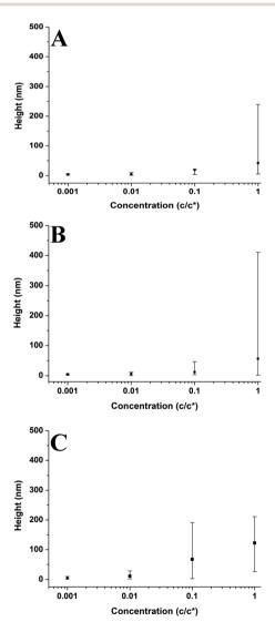
**Fig. 6** Graphs showing how concentration affects the height of the polymer aggregates on the mica surface at varying molecular weights. Each graph presents the average values and has bars which indicate the range of values. (A)  $M_n = 46 \text{ kg mol}^{-1}$ , (B)  $M_n = 86 \text{ kg mol}^{-1}$ , (C)  $M_n = 355 \text{ kg mol}^{-1}$ .
