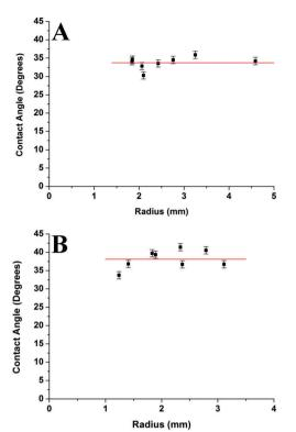
Fig. 15 Graphs showing the droplet radius against contact angle for macroscopic poly(styrene-co-butadiene) droplets at varying molecular weights on a mica surface. Measurements were taken 1 week after the samples were removed from the oven. Each horizontal line represents the overall average value of the measurements. The bars on the graphs represent the experimental error. (A)  $M_n = 46 \text{ kg mol}^{-1}$ , (B)  $M_n = 86 \text{ kg mol}^{-1}$
