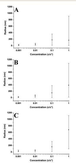
**Fig. 5** Graphs showing how concentration affects the radius of the polymer aggregates on the mica surface at varying molecular weights. Each graph presents the average values and has bars which indicate the range of values. (A)  $M_n = 46 \text{ kg mol}^{-1}$ , (B)  $M_n = 86 \text{ kg mol}^{-1}$ , (C)  $M_n = 355 \text{ kg mol}^{-1}$ .
