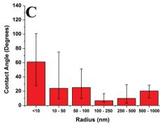
Fig. 14 Graphs showing the radius against contact angle for the nanodroplets on a mica surface at varying molecular weights. Each graph presents the average values and has bars which indicate the range of values. (A)  $M_n = 46 \text{ kg mol}^{-1}$ , (B)  $M_n = 86 \text{ kg mol}^{-1}$ , (C)  $M_n = 355 \text{ kg mol}^{-1}$ .
