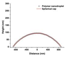
**Fig. 4** A typical cross-sectional profile plot of a poly(styrene-*co*-butadiene) random copolymer nanodroplet fitted to a spherical cap.
