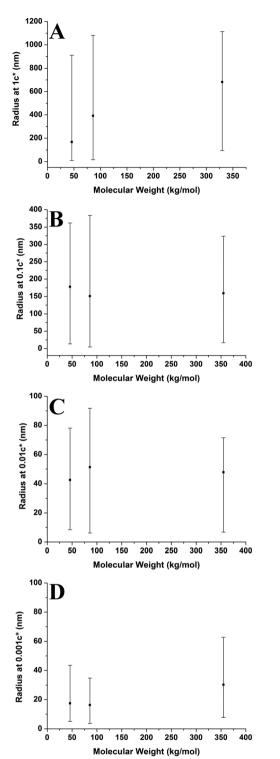
Fig. 9 Graphs showing how molecular weight affects the radius of the polymer aggregates on the mica surface at varying concentrations. Each graph presents the average values and has bars which indicate the range of values. (A) 1c\*, (B) 0.1c\*, (C) 0.01c\*, (D) 0.001c\*.
