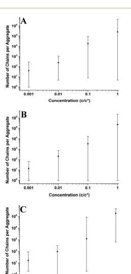
Fig. 7 Graphs showing how concentration affects the number of chains per aggregate on the mica surface at varying molecular weights. Each graph presents the average values and has bars which indicate the range of values. (A)  $M_n = 46 \text{ kg mol}^{-1}$ , (B)  $M_n = 86 \text{ kg mol}^{-1}$ , (C)  $M_n = 355 \text{ kg mol}^{-1}$ .
