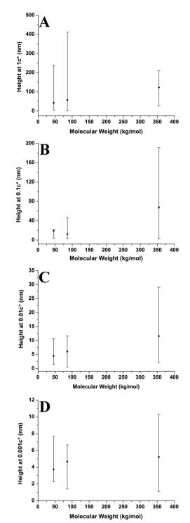
Fig. 10 Graphs showing how molecular weight affects the height of the polymer aggregates on the mica surface at varying concentrations. Each graph presents the average values and has bars which indicate the range of values. (A) 1c\*, (B) 0.1c\*, (C) 0.01c\*, (D) 0.001c\*.
