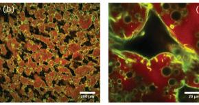
Fig. 3 (a) A mosaic of four confocal micrographs taken close together and aligned afterwards to show the morphology on a several millimeter scale. The green is the FITC labeled nanoparticles and red is the Nile Red labeled glycerol. (b and c) Confocal micrographs of a sample showing silicone oil droplets inside the glycerol phase at different magnifications where the FITC labeled nanoparticles are colored green and the Nile Red labeled glycerol is colored red
