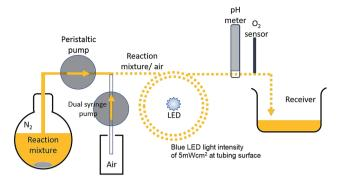
Scheme 1 Flow system set-up for continuous photo-catalysed water oxidations using  $[Ru(bpy)_3]^{2+}$ ,  $[Co(NH_3)_5Cl]Cl_2$  and  $Co_3O_4$  catalyst in 350 ml of  $N_2$  degassed 50 mM acetate buffer at pH 5.2. Illumination of 5 mW cm<sup>2</sup> at the surface of 60 cm of coiled section of tubing which contained 0.022 cm<sup>3</sup> sections of reaction mixture separated by air gaps pumped at 750  $\mu$ l min<sup>-1</sup>. pH and approximate elevation of  $O_2$  levels were recorded.
