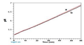
Fig. 3 (a) Graph of released  $O_2$  (µmol) against time for a photocatalytic system using  $Co_3O_4$  as catalyst and light using repeated light on : off cycles (s : s) of (a) continuous; (b) 24 : 2. (b) Graph of pH change for  $Co_3O_4$  reaction systems using repeated light on : off cycles (s : s) of (a) continuous; (b) 24 : 2.
