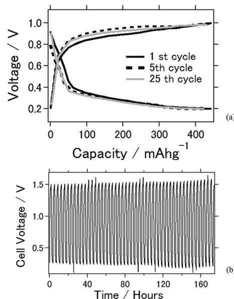
Fig. 2 (a) Charge–discharge curves of the aluminum–air battery with the TiC air cathode material at an applied current of  $\pm 0.5 \text{ mA cm}^{-2}$ . (b) Voltage *versus* time plot of the aluminum–air battery with the TiC air cathode material at an applied current of  $\pm 2.0 \text{ mA cm}^{-2}$ .
