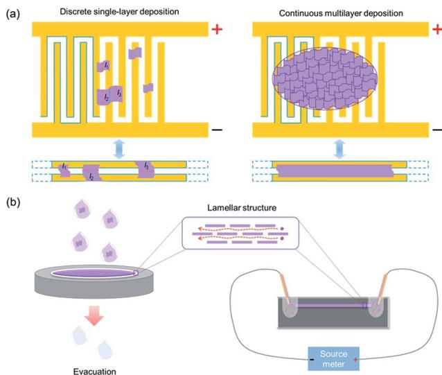
Fig. 2 Schematic diagrams for  $\text{H}^+/\text{OH}^-$  ion conductivity measurements in the case of 2D materials. (a) Comb-like microelectrode assisted measurement and (b) lamellar membrane assisted measurement.
