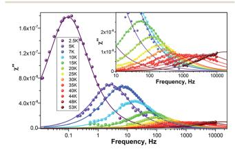
Fig. 7  $\chi''$  of Dy<sub>2</sub>S@C<sub>82</sub>-C<sub>s</sub> measured at different temperatures as a function of AC frequency. Dots are experimental points, lines are results of the fit with a generalized Debye model.
