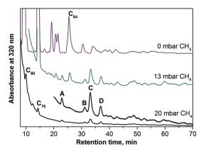
Fig. 1 HPLC traces of the extracts obtained in the arc-discharge synthesis with  $Dy_2S_3$  and different amounts of methane in the reactor atmosphere. Block letters in the lower trace denote the main clusterfullerene fractions, corresponding to (A)  $Dy_2S@C_{72}$ , (B)  $Dy_3N@C_{80}$ , (C)  $Dy_2S@C_{82}$ -I/ $Dy_2C_2@C_{82}$ -I, and (D)  $Dy_2S@C_{82}$ -II. Note that a different intensity is used for each curve.
