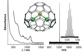
Fig. 4 UV-vis-NIR absorption spectrum (left) and positive-ion LDI mass-spectrum (right) of Dy<sub>2</sub>S@C<sub>72</sub>. The molecular structure of Dy<sub>2</sub>S@C<sub>72</sub>- $C_s$ (10528) is shown in the middle, and adjacent pentagon pairs are highlighted in black.
