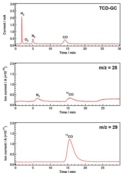
Fig. 2 Gas chromatogram and mass spectra ( $m/z = 28$  and  $29$ ) obtained during the photocatalytic conversion of  $^{13}\text{CO}_2$  using Ag-modified  $\text{Sr}_{1.6}\text{K}_{0.35}\text{Na}_{1.45}\text{Ta}_5\text{O}_{15}$ . Amount of catalyst: 0.5 g; cocatalyst loading: 5.0 wt% Ag; light source: 400 W high-pressure Hg lamp; water volume: 1.0 L;  $\text{CO}_2$  flow rate:  $30 \text{ mL min}^{-1}$ ; additive: 0.5 M  $\text{NH}_4\text{HCO}_3$ .
