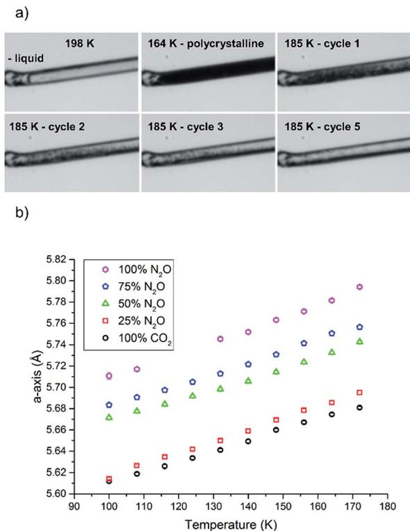
Fig. 4 (a) Condensing and annealing crystallisation of 50 : 50 mixture of CO<sub>2</sub>/N<sub>2</sub>O; cycle 4 was omitted as it did not show a substantial visual change from cycle 3. (b) Unit cell parameters for various ratios of solid solutions as a function of temperature.
