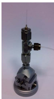
Fig. 3 A photograph of the gas cell used in the low temperature experiment.
