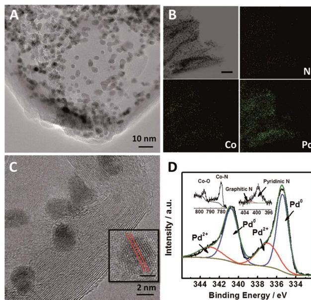
Fig. 1 Structural and elemental analysis of Pd<sub>2.2</sub>/Co–N/carbon. (A) TEM image of Pd<sub>2.2</sub>/Co–N/carbon. (B) Corresponding elemental mappings of Pd<sub>2.2</sub>/Co–N/carbon (scale bar: 50 nm). (C) HR-TEM image of Pd<sub>2.2</sub>/Co–N/carbon. The scale bar in the inset of (C) is 1 nm. (D) XPS spectra of Pd 3d, Co 2p and N 1s orbitals of Pd<sub>2.2</sub>/Co–N/carbon.
