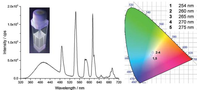
Fig. 5 Fluorescence emission spectra ( $\lambda_{\text{ex}} = 270 \text{ nm}$ ) and CIE-1931 chromaticity diagram for  $\text{tdt}[\text{Eu}(\text{EDTA})]_{0.3}[\text{Tb}(\text{EDTA})]_{2.7}$  in methanol as a function of the excitation wavelength;  $[\text{tdt}] = 25 \mu\text{M}$  and  $\chi_{\text{Eu}} = 0.1$ . Inset shows the corresponding photograph obtained with  $\lambda_{\text{ex}} = 270 \text{ nm}$ .
