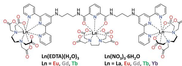
Fig. 1 Structural formula of multidentate **tdt** ligand composed of dpa and two tpy units free for binding Ln(EDTA)·(H<sub>2</sub>O)<sub>3</sub> or Ln(NO<sub>3</sub>)<sub>3</sub>·6H<sub>2</sub>O.
