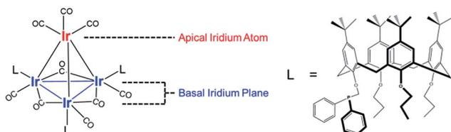
Fig. 1 Schematic representation of a trisubstituted tetrairidium carbonyl cluster, closed cluster **1** (Ir<sub>4</sub>(CO)<sub>9</sub>L<sub>3</sub>), with three bulky phosphine ligands on the basal plane of the tetrahedron (left); structure of calix[4]-arene phosphine ligand L shown at right.
