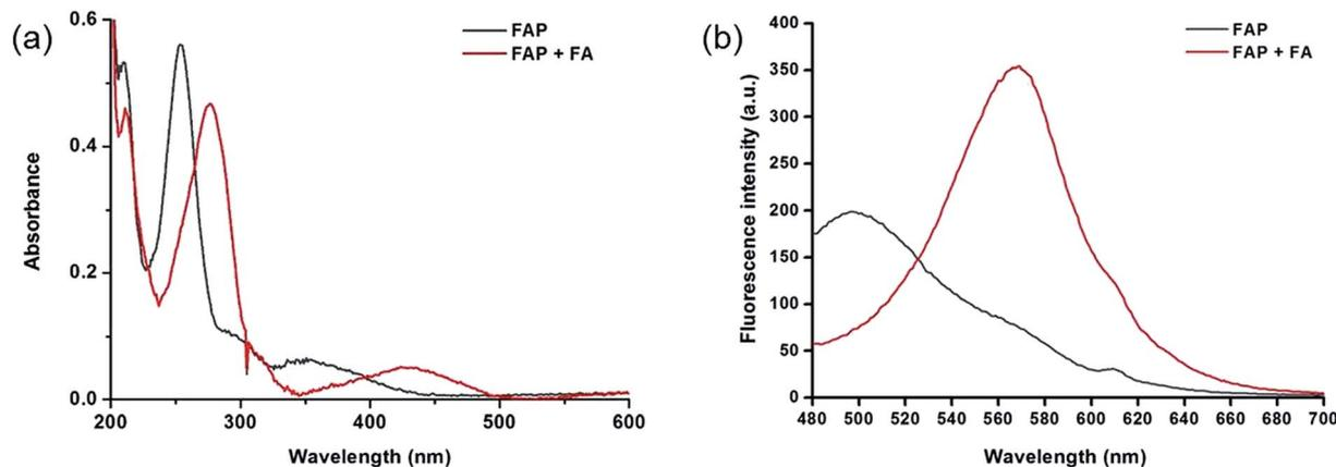
Fig. 1 (a) UV-vis absorption spectra of FAP (20  $\mu\text{M}$ ) in the absence or presence of FA (1 mM) in PBS buffer (10 mM, pH 7.4, containing 1% MeCN) at 37  $^{\circ}\text{C}$  for 120 min. (b) Fluorescence spectra of FAP (20  $\mu\text{M}$ ) in the absence or presence of FA (1 mM) in PBS buffer (10 mM, pH 7.4, containing 1% MeCN) at 37  $^{\circ}\text{C}$  for 120 min, with excitation at 405 nm, and excitation and emission slit widths = 5 nm.
