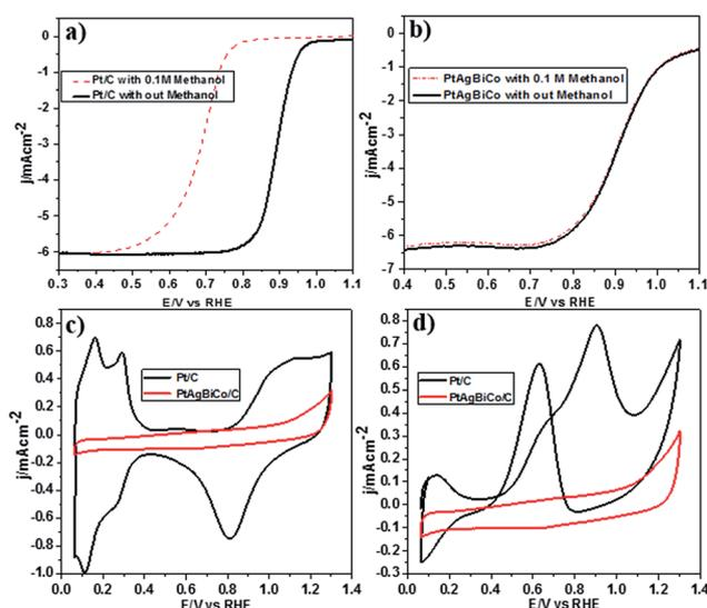
Fig. 4 ORR polarization curves for (a) Pt/C catalyst with and without 0.1 M methanol, (b) PtAgBiCo/C catalyst in O<sub>2</sub>-saturated solution with and without 0.1 M HClO<sub>4</sub> at a rotation rate of 1600 rpm. CV curve of Pt/C catalyst and PtAgBiCo/C catalyst in N<sub>2</sub>-saturated (c) 0.1 M HClO<sub>4</sub>, and (d) 0.1 M HClO<sub>4</sub> + 0.1 M CH<sub>3</sub>OH.
