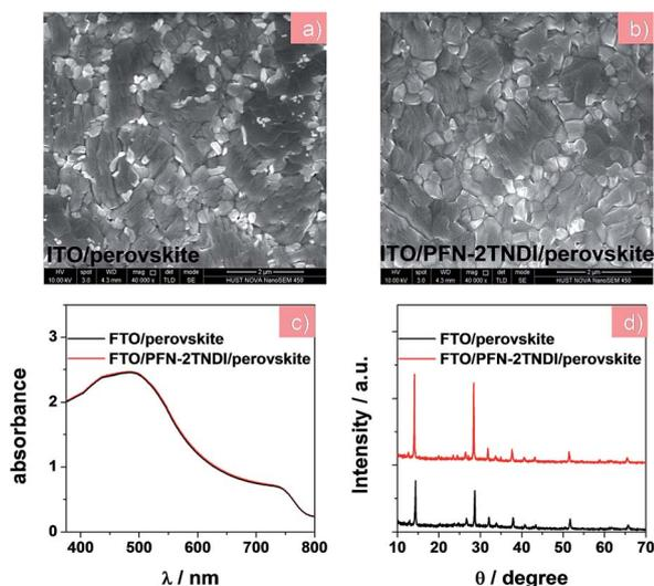
Fig. 2 (a) and (b) SEM images, (c) UV-visible absorption spectra, (d) XRD patterns of MAPbI<sub>3-x</sub>Cl<sub>x</sub> films on the ITO and ITO/PFN-2TNDI substrates, respectively.
