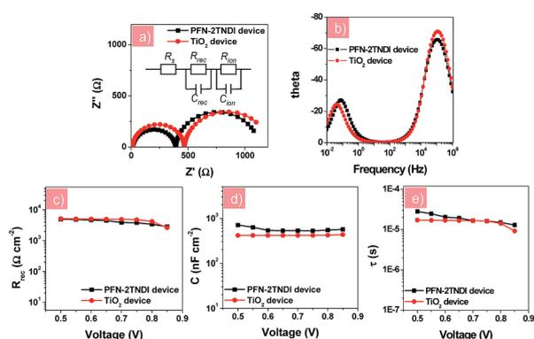
Fig. 4 (a) Nyquist plots and (b) Bode plots of perovskite solar cells with different electron transport layers; (c) the recombination resistance *R*<sub>rec</sub>; (d) the capacitance (*C*) and (e) recombination lifetime (*τ*) derived from the high frequency region as a function of the applied voltage.
