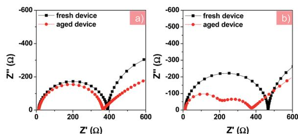
Fig. 6 Nyquist plots of fresh and aged devices based on PFN-2TNDI (a) and  $TiO_2$  (b) under illumination at a bias of  $-0.7$  V. The aged devices were under exposure to constant UV light in an argon-filled glove box for 200 h before testing.
