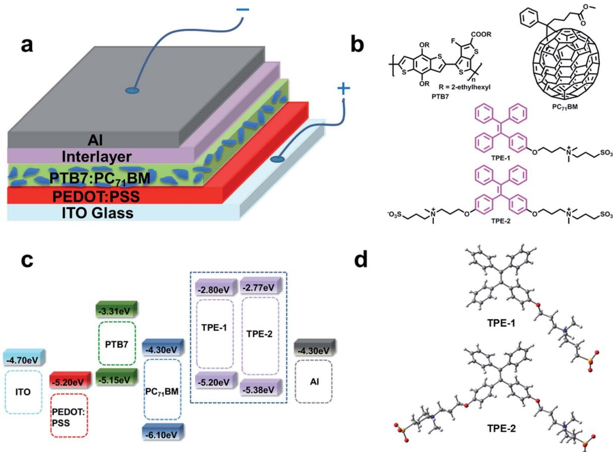
Fig. 1 (a) The device architecture. (b) Structures of the TPE derivative interlayers, PC<sub>71</sub>BM and PTB7. (c) Energy level diagram. (d) Optimized structures of TPE-1 and TPE-2.
