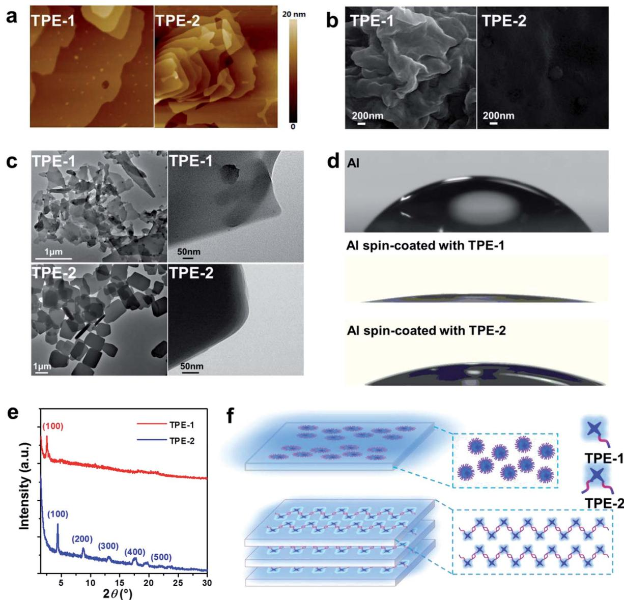
Fig. 3 (a) AFM ( $5 \times 5 \mu\text{m}$ ) images of the TPE-1 and TPE-2 films. (b) SEM images of the TPE-1 and TPE-2 films. (c) TEM images of the micro-particles of TPE-1 and TPE-2. (d) Contact angles of the aluminum films in the presence/absence of the TPE-1 or TPE-2 film. (e) GIXRD pattern of the TPE-1 and TPE-2 films on a silicon substrate (out-of-plane). (f) Abridged general view of the possible aggregate state of TPE-1 and TPE-2 in the film state.
