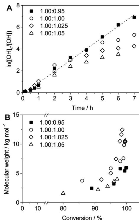
Fig. 1 (A) Kinetic plot of  $\ln([\text{OH}]_0/[\text{OH}])$  vs. time, for step-growth polymerization of 1,6-hexanediol 3a and 2b in four different ratios using 5 mol% CsF in EtOAc, as obtained from <sup>1</sup>H-NMR. Dashed line represent linear fit to (■),  $R^2 = 0.99$ . (B) Plots of  $M_n$  vs. monomer conversion, as obtained from <sup>1</sup>H-NMR and SEC.
