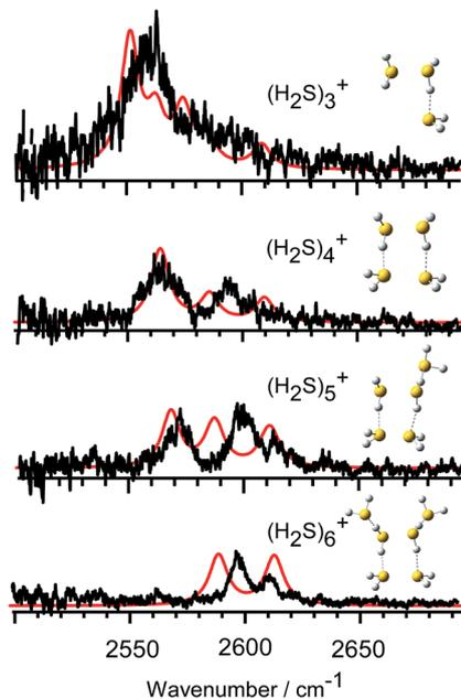
Fig. 3 Comparison between the observed spectra and harmonic spectra of the most stable isomers of  $(\text{H}_2\text{S})_n^+$  ( $n = 3-6$ ) in the free SH region. The simulation was performed at the UMP2/aug-cc-pVDZ level of theory with a scaling factor of 0.942.
