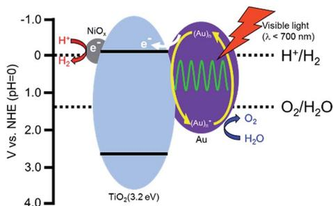
Scheme 1 Expected reaction mechanism for the production of  $\text{H}_2$  and  $\text{O}_2$  from water over a  $\text{Au}/\text{TiO}_2\text{-NiO}_x$  sample.
