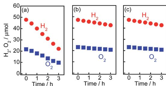
Fig. 5 Water formation from H<sub>2</sub> and O<sub>2</sub> in the dark on (a) Au(1.0)/TiO<sub>2</sub>-Pt(0.5), (b) Au(1.0)/TiO<sub>2</sub>-NiO<sub>x</sub>(0.5) and (c) Au(1.0)/TiO<sub>2</sub> samples. This experiment was carried out in pure water (300 cm<sup>3</sup>) using a closed-gas circulation system containing a stoichiometric mixture of H<sub>2</sub> and O<sub>2</sub> gases.
