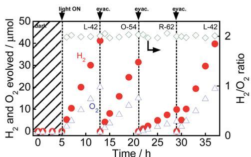
**Fig. 7** Time courses of evolution of H<sub>2</sub> and O<sub>2</sub> from water over Au(1.0)/TiO<sub>2</sub>-NiO<sub>x</sub>(0.5) under irradiation of visible light from a Xe lamp with various filters. After 13, 21 and 29 h of irradiation and evacuation, the suspension was irradiated again.
