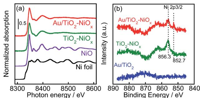
Fig. 4 (a) Ni K-edge XANES spectra of Ni foil, NiO,  $\text{TiO}_2\text{-NiO}_x(0.5)$  and  $\text{Au}(1.0)/\text{TiO}_2\text{-NiO}_x(0.5)$ ; (b) XPS spectra of  $\text{Au}(1.0)/\text{TiO}_2$ ,  $\text{TiO}_2\text{-NiO}_x(0.5)$  and  $\text{Au}(1.0)/\text{TiO}_2\text{-NiO}_x(0.5)$  around Ni 2p components.
