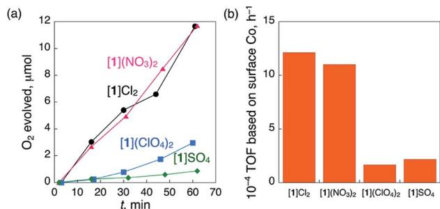
Fig. 3 (a) Time-dependent profiles of the evolution of O<sub>2</sub> during treatment with a catalytic amount of 1.0 × 1.0 × 1.0 mm-sized crystals of [1]Cl<sub>2</sub> (5.2 mg), [1](NO<sub>3</sub>)<sub>2</sub> (5.1 mg), [1](ClO<sub>4</sub>)<sub>2</sub> (4.8 mg) or [1]SO<sub>4</sub> (5.3 mg) with 5% aqueous H<sub>2</sub>O<sub>2</sub> (1.00 mL) at 298 K and (b) TOF calculated based on the number of surface Co atoms at 15 min.
