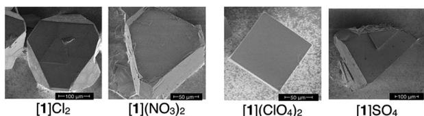
Fig. 4 SEM images of crystals [1]Cl<sub>2</sub>, [1](NO<sub>3</sub>)<sub>2</sub>, [1](ClO<sub>4</sub>)<sub>2</sub>, and [1]SO<sub>4</sub>.
