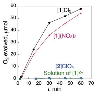
Fig. 2 Time-dependent profiles of the evolution of  $\text{O}_2$  during treatment with a catalytic amount of  $[1]\text{Cl}_2$  (5.0 mg),  $[1](\text{NO}_3)_2$  (4.9 mg),  $[2]\text{ClO}_4$  (5.0 mg) and a homogeneous saturated solution of  $[1]\text{Cl}_2$  in  $\text{H}_2\text{O}$  (0.83 mL) with 5% aqueous  $\text{H}_2\text{O}_2$  (1.00 mL total) at 298 K.
