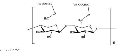
Fig. 1 Chemical structure of CMC.
