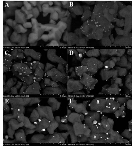
Fig. 2 SEM images of  $\text{Li}_4\text{Ti}_5\text{O}_{12}/\text{Ag}-\text{Cu}$  composites: (A) 0%, (B) 1%, (C) 2%, (D) 3%, (E) 4%, (F) 5% wt Ag-Cu.
