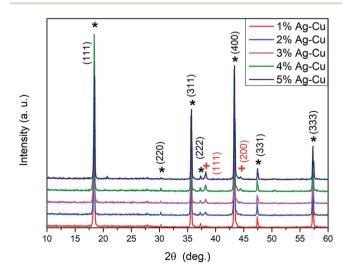
Fig. 1 XRD patterns of  $\text{Li}_4\text{Ti}_5\text{O}_{12}/\text{Ag}-\text{Cu}$  composites (\*  $-\text{Li}_4\text{Ti}_5\text{O}_{12}$ , + -Ag).
