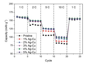
Fig. 9 Rate capability of Li<sub>4</sub>Ti<sub>5</sub>O<sub>12</sub>/Ag-Cu composites
