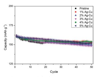
Fig. 7 Cyclability of  $Li_4Ti_5O_{12}/Ag-Cu$  composites.
