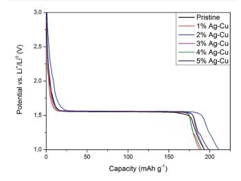
Fig. 5 Initial discharge curves of  $\rm Li_4Ti_5O_{12}/Ag-Cu$  composites during cyclability tests.
