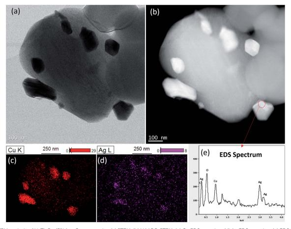
Fig. 3 STEM analysis of Li<sub>4</sub>Ti<sub>5</sub>O<sub>12</sub>/5% Ag-Cu composite: (a) STEM, (b) HAADF-STEM, (c) Cu EDS mapping, (d) Ag EDS mapping, (e) EDS spectrum of the area circled in red
