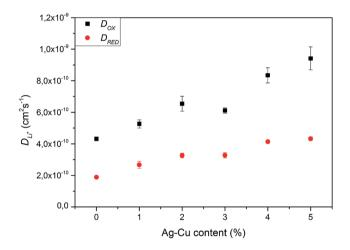
Fig. 13 Li<sup>+</sup> chemical diffusion coefficient values calculated from CV experiments of Li<sub>4</sub>Ti<sub>5</sub>O<sub>12</sub>/Ag–Cu composites.
