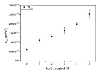
Fig. 16 Li<sup>+</sup> chemical diffusion coefficient values calculated from EIS spectra of Li<sub>4</sub>Ti<sub>5</sub>O<sub>12</sub>/Ag-Cu composites.
