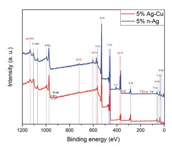
Fig. 4 XPS spectra of  $\rm Li_4Ti_5O_{12}/5\%$  Ag-Cu and  $\rm Li_4Ti_5O_{12}/5\%$  n-Ag composites.
