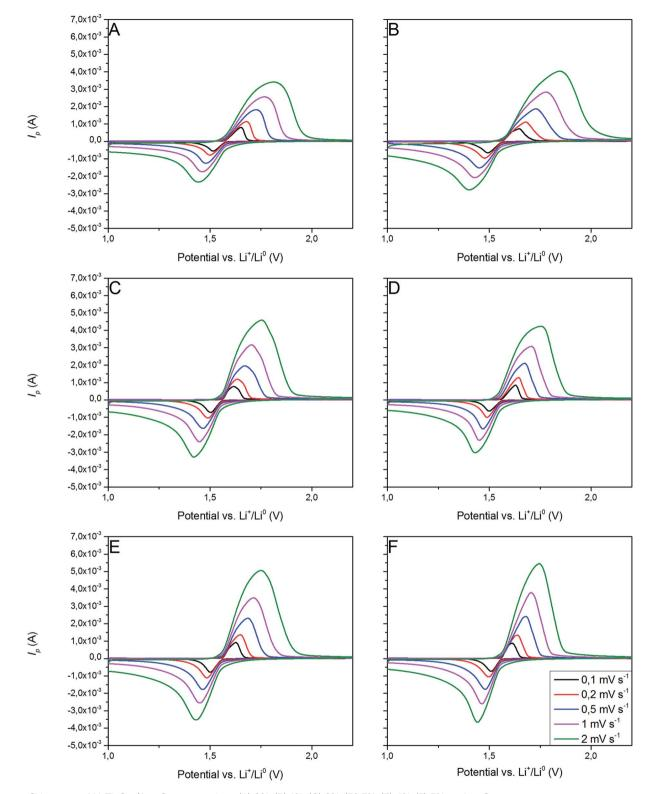
Fig. 11 CV curves of  $\text{Li}_4\text{Ti}_5\text{O}_{12}/\text{Ag}-\text{Cu}$  composites: (A) 0%, (B) 1%, (C) 2%, (D) 3%, (E) 4%, (F) 5% wt Ag-Cu.
