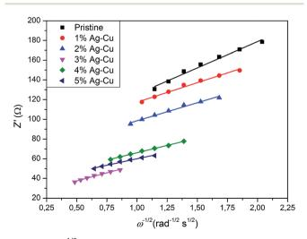
Fig. 15  $Z'(\omega^{-1/2})$  relationship acquired from EIS experiments of Li<sub>4</sub>Ti<sub>5</sub>O<sub>12</sub>/Ag-Cu composites.
