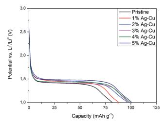
Fig. 10 Discharge curves of  $Li_4Ti_5O_{12}/Ag$ -Cu composites at 10C rate
