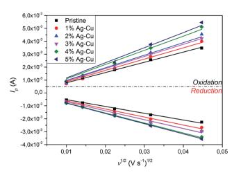
Fig. 12  $I_p(v^{-1/2})$  relationship acquired from CV curves of Li<sub>4</sub>Ti<sub>5</sub>O<sub>12</sub>/Ag–Cu composites.
