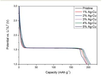
Fig. 8 Initial discharge curves of  $\rm Li_4Ti_5O_{12}/Ag-Cu$  composites during high-rate tests.
