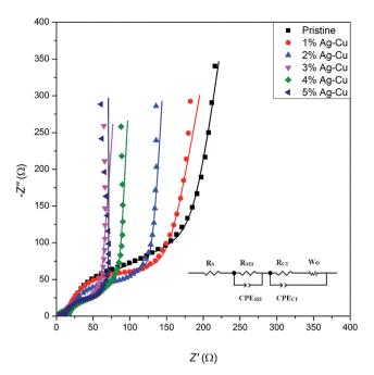
Fig. 14 Complex plane plots of  $\rm Li_4Ti_5O_{12}/Ag-Cu$  composites. Inset shows the equivalent circuit used for data fitting.
