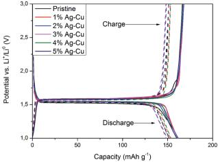
Fig. 6 Charge/discharge curves for  $\rm Li_4Ti_5O_{12}/Ag-Cu$  composites during cyclability tests: solid line –  $\rm 1^{st}$  cycle, dashed line –  $\rm 50^{th}$  cycle.
