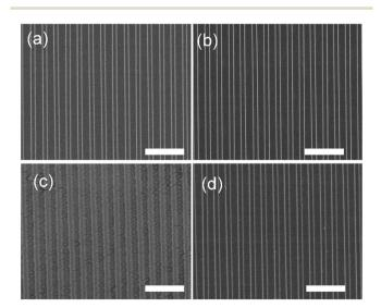
Fig. 5 SEM images of PDMS gratings. SEM of (a) (1:10) PDMS grating surface, (b) CD piece used to prepare (1:10) PDMS grating, (c) (1:35) PDMS surface, and (d) CD piece used to prepare (1:35) PDMS grating. The (1:10) PDMS (a) is copied with high fidelity when compared to the CD template. The (1:35) PDMS (c) copies the CD pattern but with some slight distortion. The scale bar is 5  $\mu$ m in all images.
