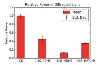
Fig. 7 Power of diffracted light from CD and PDMS samples. The power of the first order diffracted beams is compared between a CD piece, a (1:10) PDMS grating, a (1:35) PDMS grating, and a platinum (Pt) coated (1:35) PDMS grating. The softer PDMS produces lower power diffracted light, however, the Pt coating appears to restore much of the intensity lost due to the softness of the (1:35) PDMS.
