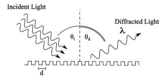
Fig. 1 Diagram of diffraction process. Incident light composed of multiple wavelengths of light undergoes diffraction when reflecting or transmitting through a repeating structure. The incident light comes in with an incident angle of  $\theta_i$  and light with wavelength  $\lambda$  is diffracted at angle  $\theta_d$ . The diffracted angle depends on the interval of the repeating structure,  $d_i$  also referred to as the grating element spacing.
