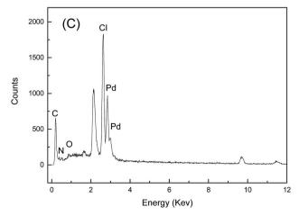
Fig. 10 SEM images of PANI-AMB (a), PANI-AMB-Pd (b), EDS curves of PANI-AMB-Pd sample (c).
