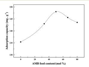
Fig. 4 Adsorption capacity of the copolymers in different AMB feed contents. (Initial Pd(II) concentration of 442.0 mg  $L^{-1}$ , T = 298 K, t =45 min).
