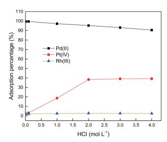
Fig. 6 Effect of HCI concentration on the selective adsorption of Pd(II) over Pt(VI) and Rh(III).
