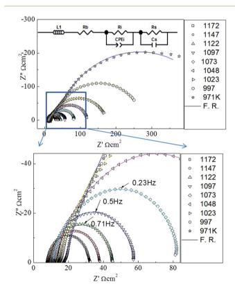
Fig. 2 The Nyquist plot of the PBCO/YSZ/PBCO symmetric cell in  $\rm CO_2$  ambient from 973 to 1173 K. The inset shows the equivalent circuit used for the fitting of the Nyquist plot. The solid lines are the fitting results.
