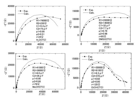
Fig. 9 The Cole-Cole plots obtained with the impedance measurements of the solution-electrode systems.
