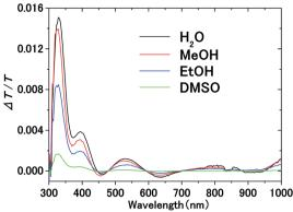
Fig. 4 Electromodulation spectra of solvents on the ITO electrode. AC voltage at frequency f is applied between the electrodes in electrolyte solution.
