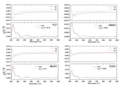
Fig. 6 Measured electromodulation spectra (black lines) and fitted spectra (red lines) with the complex refractive index change  $\Delta n + i\Delta k$  in the space charge layer of the ITO electrode shown above and the constant refractive index change  $\Delta n_s$  in the electric double layer of the solution.
