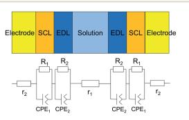
Fig. 8 Equivalent circuit for the measured system, which consists of interfacial layers, the bulk electrode, and the bulk solution. Since the two electrodes are equivalent, the circuit parameters are the same.
