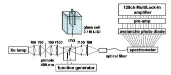
Fig. 2 Experimental setup.
