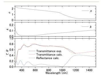
Fig. 3 Transmittance of the ITO substrate in air and the complex refractive index fitted to the experimental transmittance.
