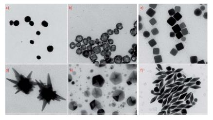
Fig. 2 TEM micrographs presenting Ag and Au nanoparticles with different geometry and shapes practically used as electromagnetic nanoresonators for SERS measurements: (a) quasi-spherical silver nanoparticles, (b) hollow spherical silver nanoparticles, (c) cubic silver nanoparticles, (d) qold-silver nanostars, (e) silver decahedral nanoparticles, (f) gold bipyramid.
