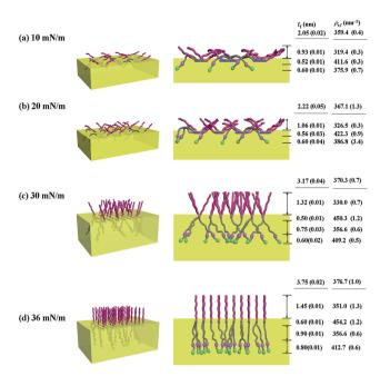
Fig. 7 Molecular models of the Langmuir films of PECH-DMAPS $_{20}$  prepared at the air-water interface under various surface pressures: (left) view with a tilt angle from the top; (right) front view along the polymer backbone.
