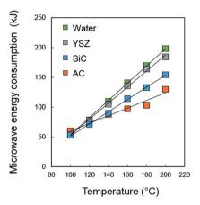
Fig. 1 Comparison of microwave energy consumption of aqueous suspension of AC (type A), SiC and YSZ under hydrothermal condition  $(100-200 \, ^{\circ}\text{C})$ .
