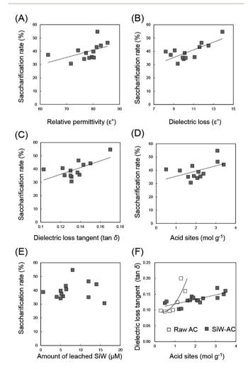
Fig. 5 Correlations among dielectric properties of AC-SiW, saccharification rate of cellobiose, acid sites and the amount of leached POM.
