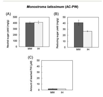
Fig. 4 Comparison of microwave (MW) and induction heating (IH) for hydrolysis of green seaweed (Monostroma latissimum) over AC-PW. (A) Neutral sugar yield, (B) reducing sugar yield and (C) amount of leached PW during reaction.
