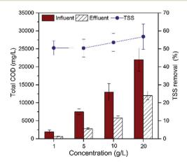
Fig. 3 Removal efficiency of total chemical oxygen demand (TCOD) and total solid suspended (TSS) removal of rMFCs fed with potato pulps waste of different organic loading rates. Error bars represent maximum deviation based on measurements from duplicate reactors in at least one month.
