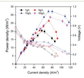
Fig. 1 Power density and polarization curves of MFCs fed with potato pulps waste of different organic loading rates. Error bars represent standard deviation based on measurements from duplicate reactors in at least three cycles.
