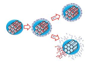
Scheme 1 Representation of the operating principle of our pH sensitive nanocarrier. A change in the pH initiates the disassembling of the self-immolative polymer allowing cargo molecules to diffuse out of the MSNs.
