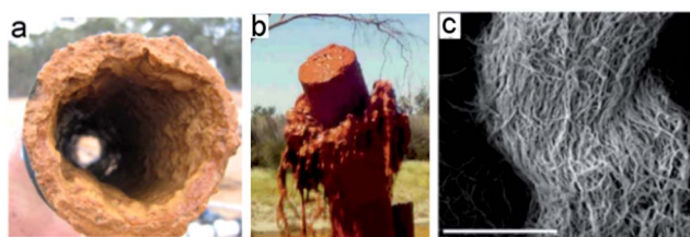
Fig. 1 (a) photo of the inside of a the pipe with the formed bacterial film with (b) cleaning process of biofilm and (c) SEM image of raw bacterial material from the biofilm (scale bar 50 µm).
