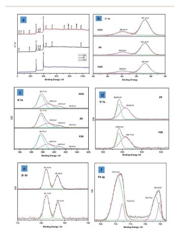
Fig. 5 XPS spectra of (a) HCN, HCN-ZR, and HCN-FZR; (b) C 1s, (c) N 1s, (d) O 1s, (e) Zr 3d, and (f) Fe 2p.
