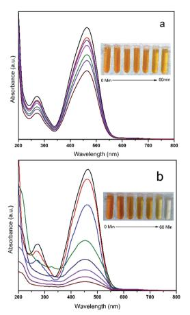
Fig. 8 UV-visible spectra. Changes in the absorbance of MO with (a) HCN-ZR and (b) HCN-FZR.
