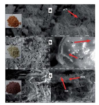
Fig. 3 SEM at different magnifications: (a) HCN, (b) HCN-ZR, (c) HCN-FZR.
