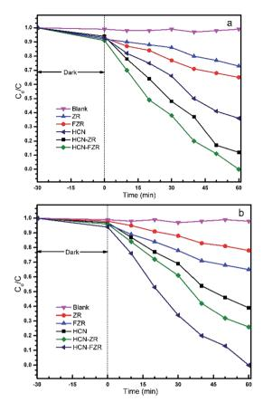
Fig. 9 Photo-catalytic degradation of (a) MTSM, and (b) MO.
