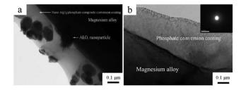
Fig. 6 TEM images of (a) PCC-Al<sub>2</sub>O<sub>3</sub> composite coating in the presence of a magnetic field of 0.3 T and (b) PCC coating in the absence of a magnetic field after 8 min of immersion in a treatment bath containing 2 g  $L^{-1}$   $Al_2O_3$  nanoparticles. (Reproduced from ref. 86, Copyright 2013, with permission from The Electrochemical Society.)
