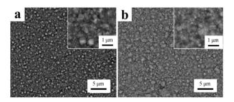
Fig. 2 Surface morphologies of (a) electroplated Ni and (b) Ni-TiO<sub>2</sub> on carbon steel. (Reproduced from ref. 56, Copyright 2010, with permission from Elsevier Ltd.)
