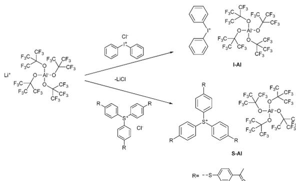
Fig. 2 Synthesis of novel diphenyliodonium and triarylsulfonium PAGs.
