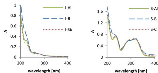
Fig. 3 Absorption spectra of diphenyliodonium and triarylsulfonium PAGs.
