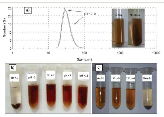
Fig. 6 Hydrodynamic size distribution and pictures of PMAO coated nanoparticles at different pH values (a, b). Pictures of the PMAO encapsulated CoFe@Pt nanoparticles in water solution at different NaCl concentrations (c). Inset is a picture of the PMAO capped nanoparticles after the surface modification of 0 and 90 days. The DLS measurements and pictures of the samples were taken after adding NaOH (a, b) and NaCl (c) for seven weeks
