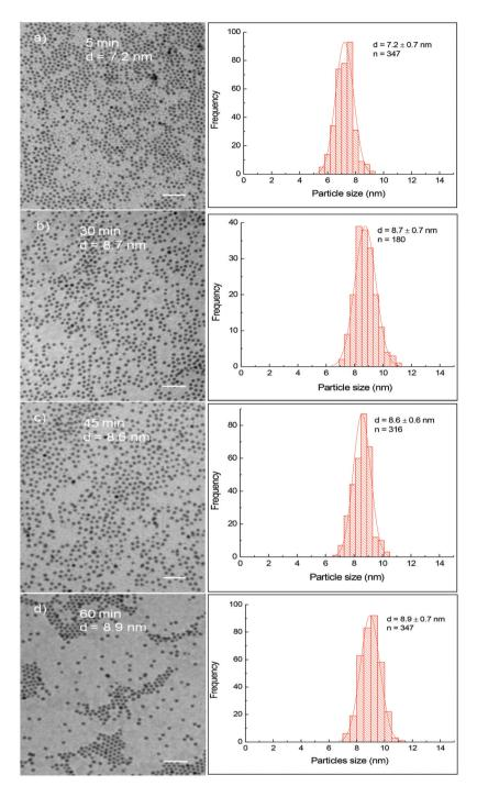
Fig. 1 TEM images and their corresponding size distribution histograms of CoFe alloy nanoparticles synthesised at different reaction times: (a) 5 min, (b) 30 min, (c) 45 nm and (d) 60 min. Scale bar: 50 nm.
