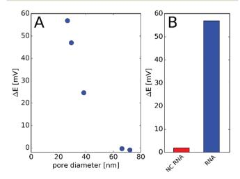
Fig. 3 (A) Potential change measured in response to 1  $\mu$ M complementary NA as a function of pore diameter and (B) response to 1 µM complementary and non-complementary (NC) miRNA with a membrane comprising an array of 7 nanopores of 26.5 nm diameter.
