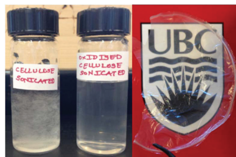
Fig. 1 Evidence of nanofibrillation achieved after oxidation of cellulose pulp using Fe@MagTEMPO as catalyst.
