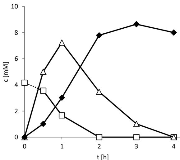
**Fig. 3** Time course of the photoenzymatic oxidation of *meso*-3-methyl-1,5-pentanediol (□) to (*S*)-4-methyltetrahydro-2*H*-pyran-2-one (◆) via the intermediate lactol (△). General conditions: 100 mM glycine-NaOH buffer (pH 9), 100 mM, [diol]<sub>0</sub> = 10 mM, [NADH]<sub>0</sub> = 1 mM, [FMN] = 100 μM, [HLADH] = 7.4 μM, 5 drops of catalase, *T* = 30 °C.
