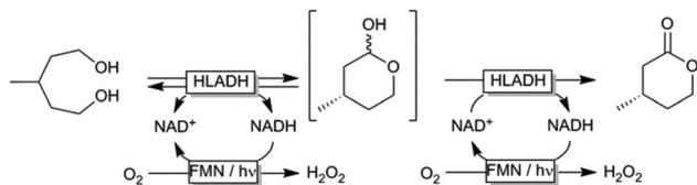
**Scheme 2** Oxidative lactonization of *meso*-3-methyl-1,5-pentanediol to (*S*)-4-methyltetrahydro-2*H*-pyran-2-one using horse liver alcohol dehydrogenase (HLADH) and photocatalytic, aerobic regeneration of NAD<sup>+</sup>.
