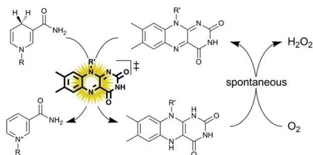
**Scheme 1** Aerobic oxidation of reduced nicotinamide cofactors (NAD(P)H) to the corresponding cofactors (NAD(P)<sup>+</sup>) using photoexcited flavin catalysts. Upon photoexcitation ( $\lambda = 450$  nm) the redox potential of the oxidised flavin catalyst increases dramatically<sup>16</sup> enabling fast hydride transfer from NAD(P)H to the flavin. The reduced flavin reacts spontaneously in a dark reaction with molecular oxygen.<sup>14</sup>
