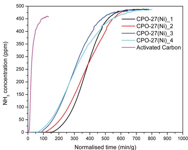
Fig. 2 Ammonia breakthrough curves for CPO-27(Ni)<sub>1</sub> to CPO-27(Ni)<sub>4</sub> and a commercial activated carbon sample.
