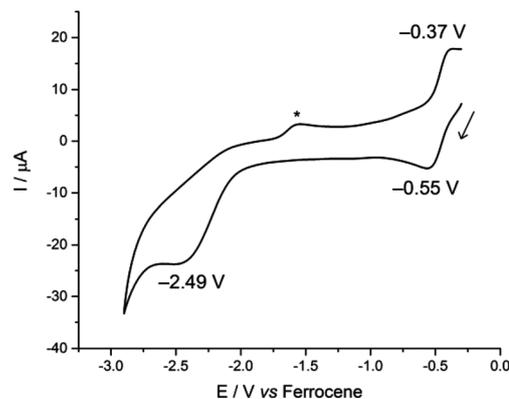
Fig. 3 Cyclic voltammogram of **3**, measured at 100 mV s<sup>–1</sup> in 0.1 M CH<sub>2</sub>Cl<sub>2</sub>/[<sup>n</sup>Bu<sub>4</sub>N][BPh<sub>4</sub>]. The asterisk denotes a decomposition product that is formed only after the irreversible reduction.
