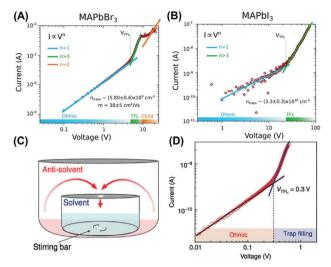
**Fig. 7** SCLC measurements of (A) MAPbBr<sub>3</sub> and (B) MAPbl<sub>3</sub> single crystals grown by an anti-solvent vapor-assisted method, and (C and D) MAPbBr<sub>3</sub> planar-integrated single-crystals. Reproduced with permission: (A and B) from ref. 29. Copyright 2015, American Association for the Advancement of Science. (C and D) From ref. 39. Copyright 2015, Nature Publishing Group.
