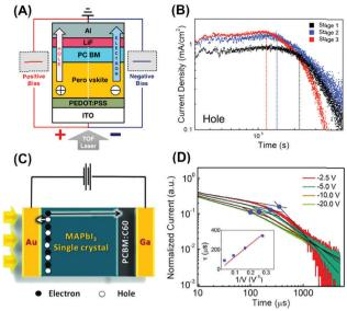
Fig. 4 Schematic TOF measurements and results of (A and B) two-step fabricated MAPbl<sub>3</sub> solar cells upon continuous light illumination and (C and D) MAPbl<sub>3</sub> single crystal based devices. Reproduced with permission: (A and B) from ref. 28. Copyright 2016, American Chemical Society. (C and D) From ref. 30. Copyright 2015, American Association for the Advancement of Science.
