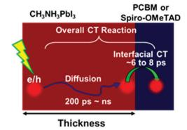
Fig. 10 Schematic illustrating charge dynamics in perovskites attached to the charge acceptor in the device configuration. Reproduced with permission from ref. 4. Copyright 2016, American Chemical Society.
