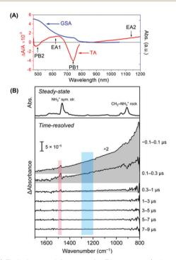
Fig. 1 (A) Typical spectral features of a TA spectrum (red curve) of an MAPbl<sub>3</sub> film directly after photoexcitation together with its ground-state absorption (GSA) spectrum (blue curve). (B) TA spectra in the near-IR region revealing the Fano resonances between the vibrational transitions of the MA cation and the quasi-continuous intra-CB transition (red region). Reproduced with permission: (B) from ref. 4. Copyright 2016, American Chemical Society
