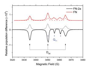
Fig. 1 X-band (9.8 GHz) CW transient EPR spectra of 1.5 mM FN (red) and FN-2a (black) in toluene recorded 2.5 μs (solid trace) and 4.1 μs (dash trace) after pulse laser excitation. Transitions assigned to the  $D_{S0}$  and  $Q_{T1}$  states are marked.
