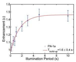
Fig. 5 Build-up of  $^1\text{H-NMR}$  signal enhancements of toluene doped with 0.8 mM **FN-1a** at different laser (2.8 W) illumination periods. The red trace is the fitted curve with a build-up time  $T_{\text{build-up}} = 1.6 \pm 0.4$  s. The  $T_{1n}$  for **FN-1a** is  $3.2 \pm 0.3$  s, the difference between  $T_{1n}$  and  $T_{\text{build-up}}$  is likely due to the heating effects.
