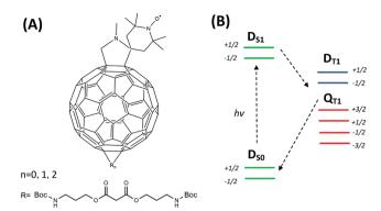
Scheme 1 (A) Scheme of the **FN** (n=0) structure and its derivatives **FN-1a** and **FN-2a** (n=1, 2) with different numbers of adducts (R). (B) Simplified energy level scheme and transitions of **FN** after laser excitation according to Corvaja & coworkers.<sup>22</sup>
