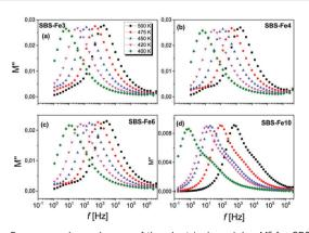
Fig. 9 Frequency dependences of the electrical modulus M" for SBS-Fe3 glass (a), SBS-Fe4 glass (b), SBS-Fe6 glass (c) and SBS-Fe10 glass (d) at selected temperatures. The data are connected as a guide to the eye.
