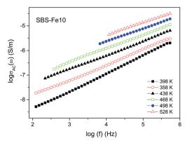
Fig. 7 Frequency dependences of the ac conductivity,  $\sigma_{AC}$ , for the glass containing 10 mol% of Fe<sub>2</sub>O<sub>3</sub> (SBS-Fe10) at selected temperatures.
