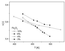
Fig. 8 Temperature dependence of the s parameter for the glasses with various contents of Fe<sub>2</sub>O<sub>3</sub>.
