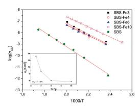
**Fig. 6** Temperature dependence of the dc conductivity,  $\sigma_{DC}$ , for various glass compositions. The solid lines represent the least-square fitting. Inset shows the variation of the  $\sigma_0$  with the concentration of Fe<sub>2</sub>O<sub>3</sub>.
