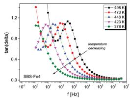
Fig. 4 Frequency dependences of the dielectric loss  $\tan\delta$  at selected temperatures for SBS-Fe4 glass. The data are connected as a guide to the eye.
