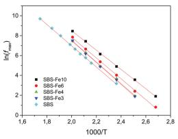
Fig. 10 Frequency dependences of the M'' peak on 1000/T for Na<sub>2</sub>O-B<sub>2</sub>O<sub>3</sub>-SiO<sub>2</sub>-Fe<sub>2</sub>O<sub>3</sub>. The data are connected as a guide to the eye.
