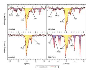
Fig. 2 Mössbauer spectra were recorded for the samples containing iron. Different regions on the graphs represent contributions from the different
