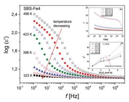
Fig. 3 Frequency dependences of the real part of the electric permittivity arepsilon' at selected temperatures for SBS-Fe4 glass. Inset (a) shows the frequency dependence of the real part of the electric permittivity at 300 K for  $Na_2O-B_2O_3-SiO_2-Fe_2O_3$  glasses ( $Fe_2O_3$  content is indicated). Inset (b) shows the variation in the real part of the electric permittivity at 1 kHz with Fe<sub>2</sub>O<sub>3</sub> concentration evaluated at selected temperatures.
