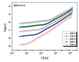
Fig. 5 Temperature dependence of the conductivity,  $\sigma$ , at several temperatures for SBS-Fe10 glass. The data are connected as a guide to the eye.
