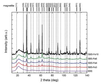
Fig. 1 XRD patterns for the  $xFe_2O_3-8Na_2O-(22-x)B_2O_3-70SiO_2$  glasses. The vertical offsets were used for clarity. The positions of reflections for the bulk magnetite are indicated
