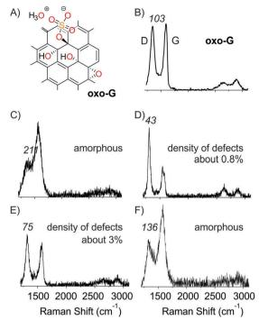
Fig. 2 (A) Chemical sketch of oxo-G. (B) Raman spectrum of oxo-G before treatment;  $\Gamma_{\rm D}$  values are given in italic numbers. (C–F) Raman spectra of electron beam irradiated areas shown in Fig. 1B at selected energies and doses. (C) 2 keV and 800 mC cm<sup>-2</sup>, (D) 30 keV 50–800 mC cm<sup>-2</sup>, (E) 2 keV and 50 mC cm<sup>-2</sup> and (F) 10 keV and 800 mC cm<sup>-2</sup>.  $\Gamma_{\rm D}$  values are given in italic numbers.
