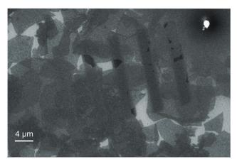
Fig. 3 Electron microscopy image recorded at 15 kV. Oxo-G flakes after irradiation (5 keV) and reduction. The electron irradiated striped areas are clearly visible as dark features. The dark features correspond to areas of reduced oxo-G by secondary electron emission and are mainly located on the bare SiO<sub>2</sub>. The observed contrast on the reduced oxo-G is likely due to modification of the underlying SiO<sub>2</sub> as well.
