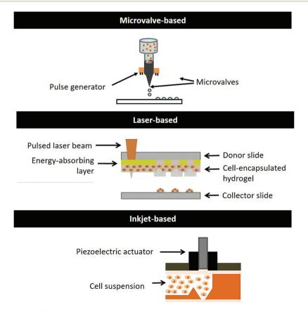
Fig. 1 Schematic drawing of different DOD bioprinting systems.
