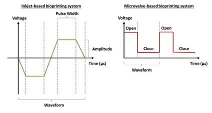
Fig. 2 Dispensing mechanisms for (left) the inkjet-based system and (right) the microvalve-based system.
