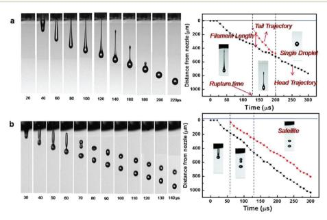
Fig. 3 (Left) Representative photo sequence of droplet formation and (right) representative trajectories of the ejected droplets as a function of the elapsed time for bio-inks with varying values of Z: (a) Z = 2.17; (b) Z = 17.32. "Reprinted (adapted) with permission from ref. 45. Copyright (2009) American Chemical Society".
