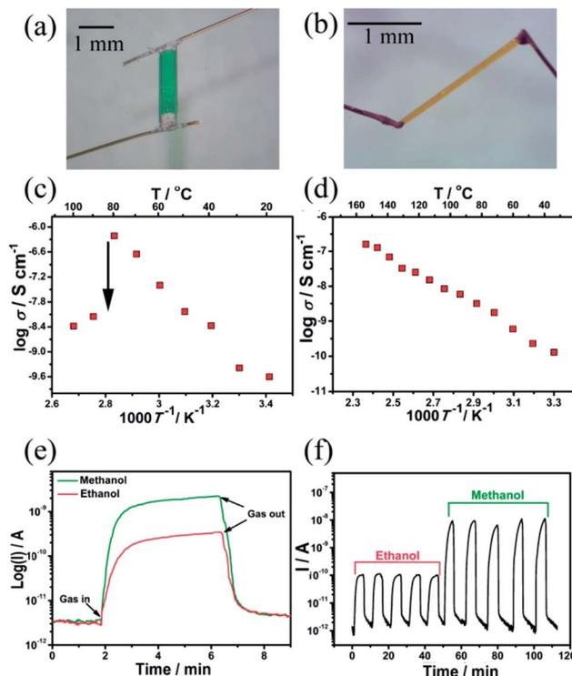
Fig. 4 Photographs of **1** (a) and **2** (b) single crystals for electronic study.  $\log \sigma$  versus temperature plot for **1** (c) and **2** (d). Room temperature gas sensitive properties of **2**: response–recovery curves of **2** to methanol and ethanol, respectively (e); repeated response of **2** to methanol and ethanol, respectively (f).
