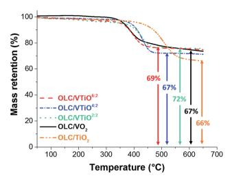
Fig. 2 Thermogravimetric analysis of all hybrid electrode samples. The measurements were carried out in synthetic air with a flow rate of 20 ml min $^{-1}$  up to a temperature of 650 °C at a heating rate of 5 °C min $^{-1}$ .
