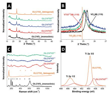
Fig. 3 (A) Survey of X-ray diffractograms of all fabricated hybrid electrodes, (B) detailed view of the (110) signal of  $OLC/VO_2$  and all multilayer hybrid samples, including the (110) reflection position of  $TiO_2(B)$ , (C) Raman spectra of all hybrid samples, including ideal peak positions of  $VO_2(M)$  and anatase, and (D) high resolution X-ray photoelectron spectra of the Ti 2p signal for hybrid samples  $OLC/TiO_2$  and  $OLC/VTiO_3^{6:2}$ .
